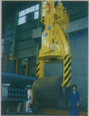
5 to 40 ton electric links-type coil lifters
